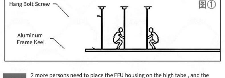
high efficiency filter should be ready for installation.
